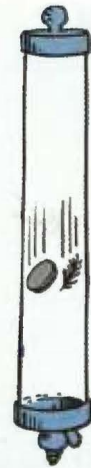
FIGURE 3.10 A feather and a coin fall at equal accelerations in a vacuum.
