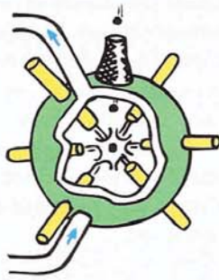
FIGURE 34.23 How laser fusion might work. Pellets of frozen deuterium are rhythmically dropped into synchronized laser crossfire. The resulting heat is carried off by molten lithium to produce steam.
