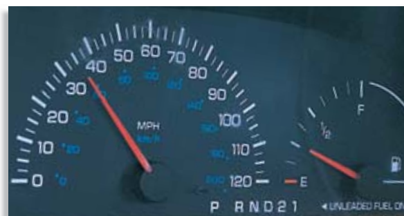
FIGURE 5 The speed that registers on a speedometer represents distance traveled per hour and is expressed in the derived units kilometers per hour or miles per hour.
