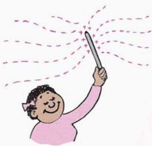
FIGURE 26.1 Shake an electrically charged object to and fro, and you produce an electromagnetic wave.
